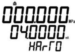
2>HART1:Display standard gauge testing current and pressure transmitter output current.
