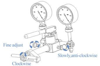
**G** Finish the loop calibration and open the relieve valve to release the pressure.
