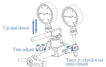
**E** Rotate the lead screw clockwise to make pressure value close to next calibration points, and adjust F-adjust valve to get exact values. Pressure rising & stabilize to 10bar, 15bar, 20bar, 25bar in turn. Meanwhile, record the data.
