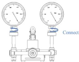
**C** Set F-adjust valve to the mid position, and for lead screw, turn all the way in.
