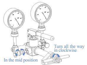
**D** Record 0bar record and close the relieve valve. Providing pressure by hand pump and leading screw let pressure near -0.2bar, then adjust the F-adjust valve to get exact pressure value.
