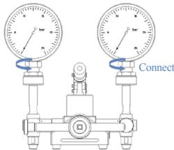
**C** Set F-adjust valve to the mid position, and for lead screw, turn all the way out.
