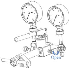
**H** Change gauge under test and calibrate the next one.
