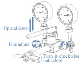
**E** Use the hand pump leading screw and F-adjust valve to calibrate other calibration point(-0.4bar,-0.6bar,-0.8bar).If the pressure value is up to -0.92bar,pls create negative pressure by turning lead screw anti-clockwise until full scale.
