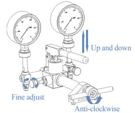
**F** Loop calibration:Turning lead screw clockwise (or together with relieve valve), and adjust the F-adjust valve to get exact values. Record the data when the pressure stabilize on -0.8bar,-0.6bar,-0.4bar, -0.2bar and so on.
