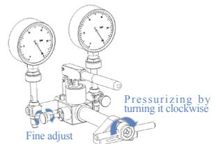
**F** Loop calibration: Decrease pressure by turning lead screw anti-clockwise (or together with relieve valve), and adjust the F-adjust valve to get exact values. Record the data when the pressure stabilize on 20bar, 15bar, 10bar, 5bar and so on.
