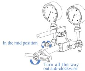
**D** Record 0bar record and close the relieve valve. Providing pressure about 4 bar by hand pump up and down, then adjust the F-adjust valve to second calibration point(5bar).
