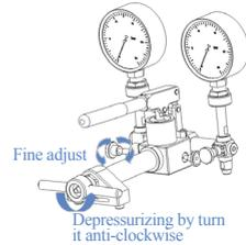
**G** Finish the loop calibration and open the relieve valve to release the pressure.
