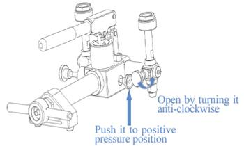
**B** Remove the plugs of outputs. Connect the standard gauge and the gauge under test to the two outputs interfaces separately, it must firm in place. Otherwise, it will be leakage.
