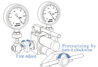
**F** Loop process: Decrease pressure by turning lead screw anti-clockwise (or together with relieve valve), and adjust the F-adjust valve to get exact values. Record the data when the pressure stabilize on 200bar, 150bar, 100bar, 50bar and so on.
