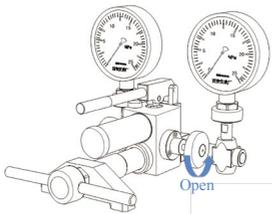
**H** Change gauge under test and calibrate next one.
