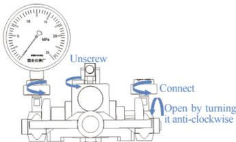
**C** Set F-adjust valve to the mid position,and for lead screw,turn all the way out.
