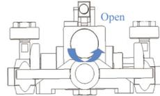
**B** Put HS705A on the level. Turn the relieve valve anti-clockwise to open it,unscrew ventilation nut.Remove the plug of the outputs,connect the standard gauge and the gauge under test to the two outputs.
