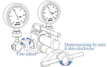
**G** Finish the loop process and open the relieve valve to release the pressure.
