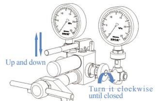
**E** Rotate the lead screw clockwise and adjust the F-adjust valve to get exact values. Pressure rising & stabilize to 50bar,100bar ,150bar,200bar,250bar in turn, meanwhile, record the data.
