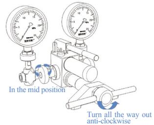
**D** Record 0bar record,and close the relieve valve:Providing pressure 20-30bar by turning hand pump up and down and stop pre-pressure.
