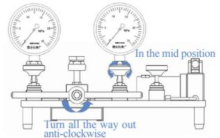
**D** Record 0bar record, and close the relieve valve: Providing pressure 20bar by turning hand pump up and down and stop pre-pressure.
