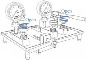
**H** Change gauge under test and calibrate next one.
