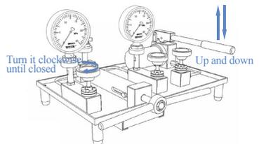
**E** Close shut-off valve clockwise. Rotate the Lead screw clockwise and adjust the F-adjust valve to get exact values. Pressure rising & stabilize to 50bar, 100bar, 150bar, 200bar, 250bar in turn, meanwhile, record the data.
