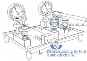
**G** Finish the loop process and open the relieve valve to release the pressure. Then open the shut-off valve.
