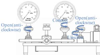
**C** Set F-adjust valve to the mid position, and for lead screw, turn all the way out.
